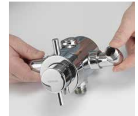
3 Adjust the Aspire valve inlet elbow centres to suit (between 148mm and 155mm)
