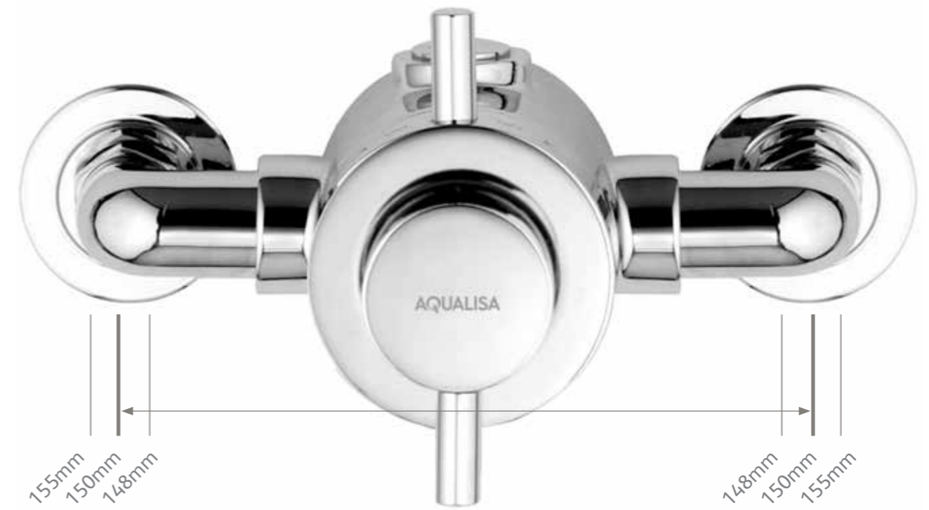
Aspire and Siren exposed valve pipe centres easily adjust from 148mm-155mm – ideal for replacing most exposed showers.
