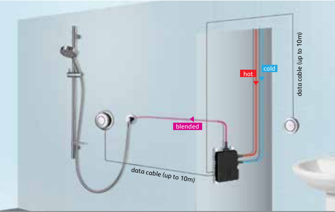
Adjustable shower Locate the remote control outside the enclosure – press the button and wait for the illuminated controls to stop flashing, and the shower will be ready by the time you’ve brushed your teeth.
