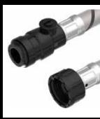
Flexible Hoses 200 mm antivibration hoses with integral isolating valves G ¾ threaded connections to pump, 15 mm push-fit to pipework
