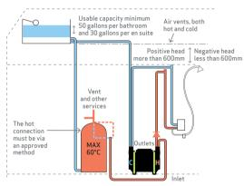
Negative head When the distance hetween the cold water storage cistern and the shower head or the highest point in the system after the pump is 600 mm or less, or when the natural flow is poor or less than 2 litres per minute (11/30 seconds hot and cold) of combined hot and cold it is possible a negative head pump may be required.
