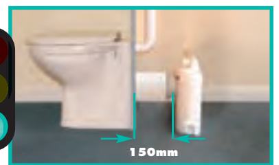
If boxed in, the boxing should be easily removed. Any extension between the WC pan spigot and wall should not exceed 150mm.
