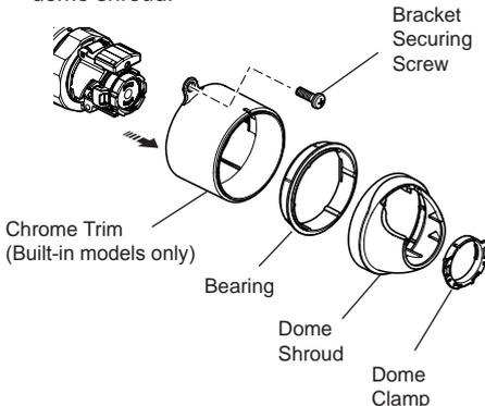
6. Remove the dome shroud, bearing and chrome trim if fitted (Built in Models only).
