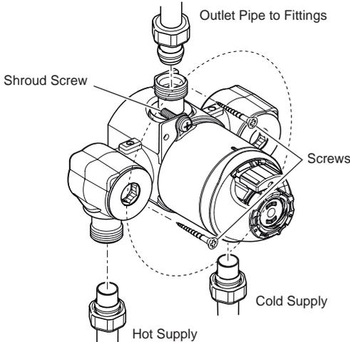
12. Connect the outlet pipework and install the RAC assembly or BIR assembly, **before** continuing with the installation of the mixing valve.
