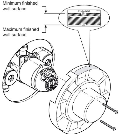
16. Remove the building-in shroud and secure the chrome trim to the mixer using two of the bracket securing screws.
