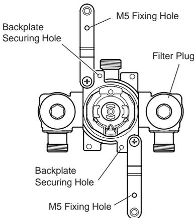
5. Drill the two  $\text{\O}5.5$  mm holes for the fixing positions (countersink the holes at the front).
