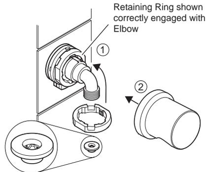
**Note!** For high pressure systems (above 0.5 bar) make sure that the flow regulator (supplied) is fitted inside the elbow in the orientation shown.
