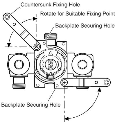
**Note!** Securing Brackets shown in preferred position to allow the Compression Nuts to be tightened.
