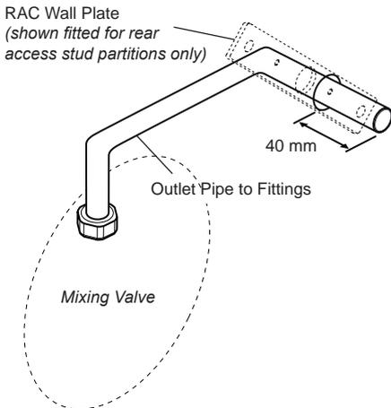
2. Temporarily cap off the outlet pipe, turn on the water supplies and check for leaks.
