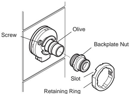
19. Check that the second 'O' seal (black) is fitted to the outside of the backplate nut. Press the elbow onto the backplate, make sure that the clips on the elbow engage with the backplate.
