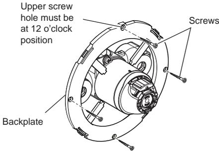
16. For solid walls drill four Ø6 mm holes for the wall plugs. For other types of wall structure alternative fixings may be required (not supplied).
