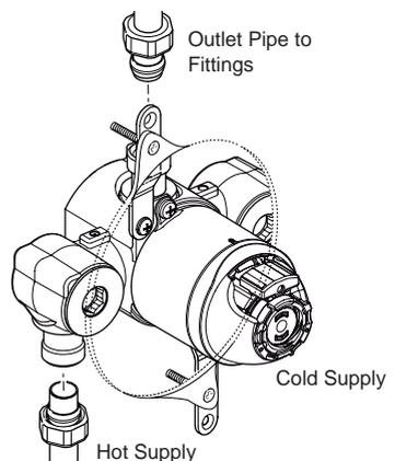
11. Turn on the water supplies and check for leaks.
