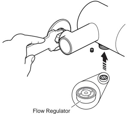
**Note!** Make sure that the flow regulator (supplied) is fitted inside the outlet nipple in the orientation shown.
