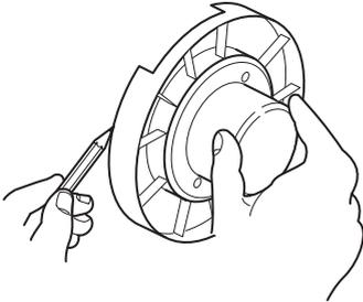
4. Mark the routes for the supply pipework at 108 mm centres (**Hot - Left, Cold - Right**).
