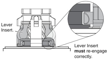
13. Make sure that the two cartridge inlet seals are fitted and carefully push the cartridge into the body, aligning the cartridge lugs into the body slots.
