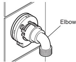
22. Slide the retaining ring over the elbow and engage with the elbow clips. **Note!** The retaining ring must be engaged correctly to lock the elbow to the backplate, rotate the retaining ring to the position illustrated.
