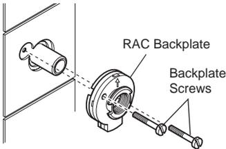
18. Check that the blue 'O' seal is fitted inside the backplate nut. Fit the olive and the backplate nut over the outlet pipe, do not tighten the nut fully at this point.
