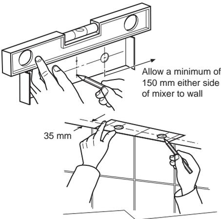
3. For solid walls drill the holes for the backplate with a 6 mm diameter drill and insert the wall plugs.
