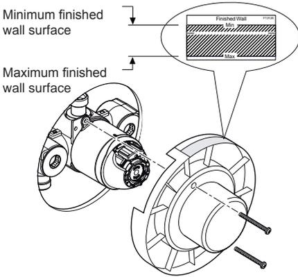
13. Using the 'Finished Wall Indicator' on the building-in shroud as a guide, finish the wall, e.g. tiles.
