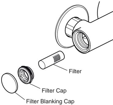
3. Clean the filters under a jet of water to remove any lodged particles.
