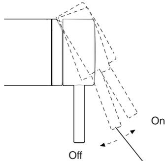
Mid Flow Override - Reduces water flow by up to 30% (dependant on inlet pressures) and can be overridden by increasing flow to full.
