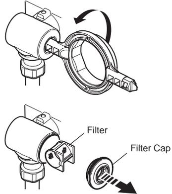
6. Clean each of the filters under a jet of water to remove any lodged particles.
