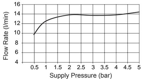
Typical flow rates on low pressure systems (0.1 to 1 Bar) without flow regulator fitted - Mira Element SLT with L14A Shower Fittings
