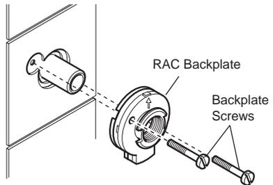
9. Loosely attach the RAC backplate to the RAC wall plate, using the two backplate screws provided.
